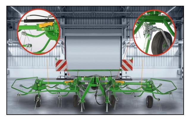
4 Rotor Carousel Tedder for tedding mowed small green plants in order to quicken the drying process. CAT II three point linkage, 540RPM.
