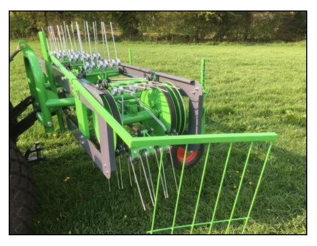
Compact hay rake which is rugged and light weight so doesn't need much horsepower to operate. Complete with three rows of double tines giving 36 double tines.
